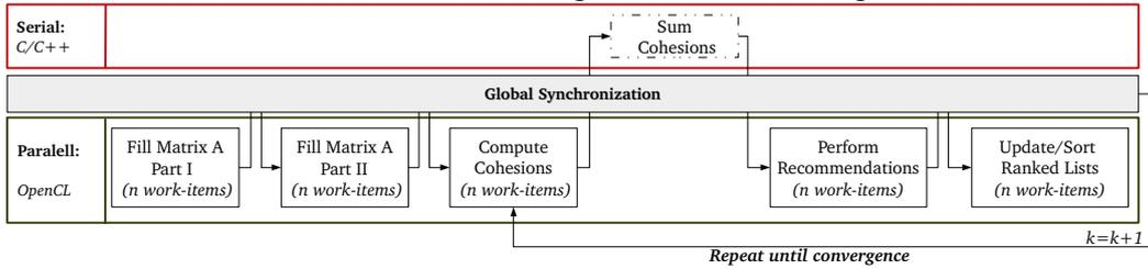
Figure 1: Design of the Parallel RL-Recommendation Algorithm.
